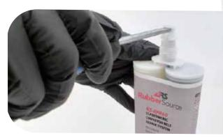
5. Screw the mixing nozzle tightly onto the cartridge.
